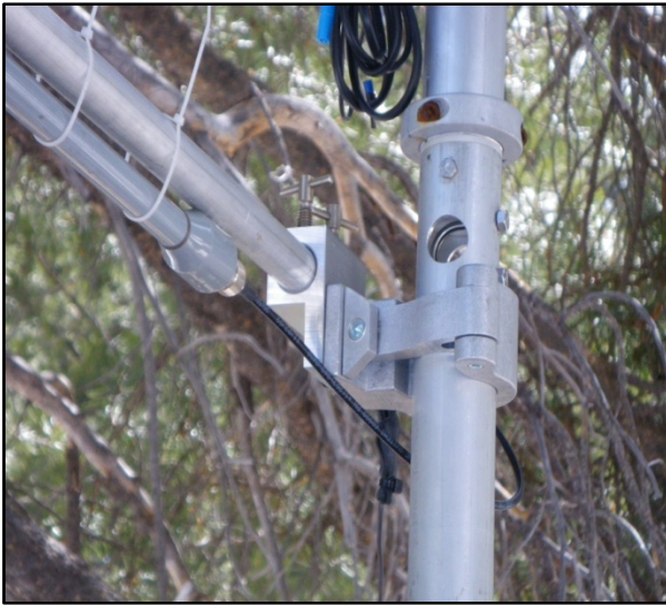
Figure 7: The adjustable calibration clamp affixed to the vertical support shaft of the Snowcloud structure.
